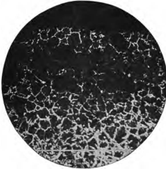
Fig. 7. Outer Portion of Case; Magnification, 50
